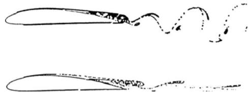
Figure 7.9: Streaklines of coarse and fine grid solutions. For meshes see figure 7.5.
